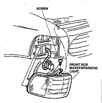
12.Unplug the connector at the front side marker/parking light, and connect the cornering lights wire harness between the two sides of the connector. Reinstall the light.
