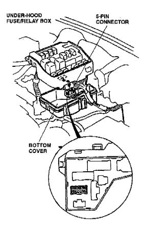
16. Route the 5-pin connectors of the cornering lights wire harness from the front bumper to the under-hood fuse/relay box; then connect the 5-pin connectors of the wire harness between the under-hood fuse/relay box and the 5-pin connector you just unplugged.
