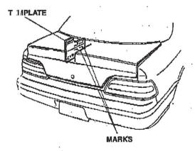
7 old the spoiler above the trunk lid, and check hat the six marks you made line up with the notes in the spoiler.
