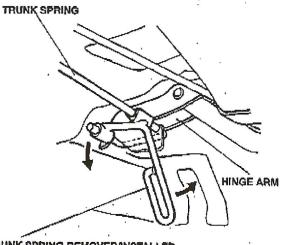
TRUNK SPRING REMOVER/INSTALLER (08M10-SM4-100) 12.Install he new rearry- uty trunk springs:
