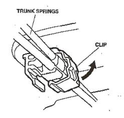
Remove the old trunk springs from the trunk hinge arms using the special tool provided. Wearing gloves, pull the tool toward you to rotate the spring.
