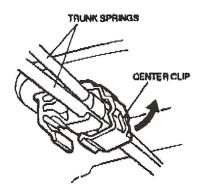
Remove the old trunk springs from the trunk hinge arms using the tool provided.
