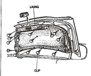
Measure 14 mm inboard from each end of the trunk lid as shown and mark that position. Draw a line through the mark in parallel with the end of the trunk lid, using a felt-tipped pen.
