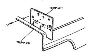
4. Hold the spoiler above the trunk lid and check that the marks made in step 3 line up with the holes of the spoiler. When you are satisfied that the marks are properly aligned, remove the spoiler and center punch each mark. Orill four 3 mm holes at the punched marks, then 6 mm holes, and finish with an 8 mm drill bit.
