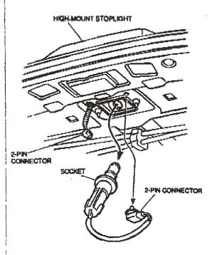
Remove the trunk room lamp. Route the stoplight harness (long-end) through the frame as shown, and plug its 2-pin connector into the 2-pin connector just unplugged. Press the tab on the 2-pin connector into the hole in the trunk panel as shown.
