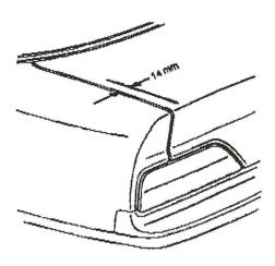
Position the template on the trunk lid along the line with the side marked "A" facing down as shown. Mark the trunk lid as indicated on the template, using a felt-tipped pen.
