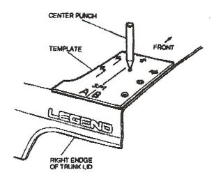
First drill a pilot hole with a 3 mm drill bit, then 6 mm, and an 8 mm, and finish with 10 mm drill bit.
